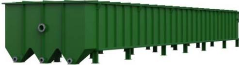
The API is the oldest of the modern gravity separator designs. This is what everyone thinks of when looking for a separator. Built to API 421 criteria its performance is <100mg/L, 150-micron free non-emulsified oil droplets. This design provides the solution for heavy solids and oil removal applications.
